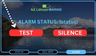
The silence button will silence the alarm buzzer, it will not stop/override a protection event from occurring. It may be used to silence the buzzer while troubleshooting. Once the alarm/protection has been cleared the buzzer will reset.
