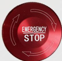
Turn emergency stop switch (pictured left) to the on position by turning clockwise in the direction of the arrows
