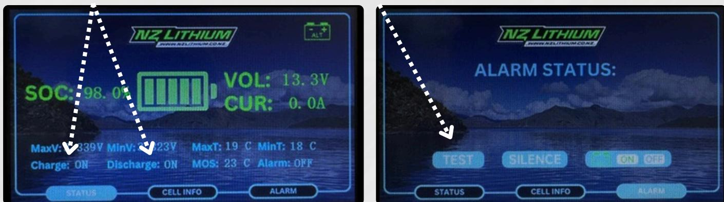
The silence button will silence the alarm buzzer, it will not stop/override a protection event from occurring. It may be used to silence the buzzer while troubleshooting. Once the alarm/protection has been cleared the buzzer will reset.
